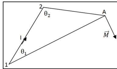
a system of  $N \times N$  linear algebraic equations is obtained. The solutions of this system are the values and the sign of the electric current intensity  $I_i$  due to  $\vec{M}_{AMB}$  and circulating on the sides of all panels approximating the external surface of the aircraft. This computation is made using a modified in house aerodynamic computer code, based on 3D vortex lattice method [5].
