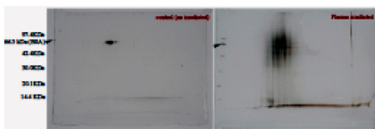
Figure 14. Before and after of nitrogen gas plasma exposure to BSA and analyzed by electrophoresis The left is before exposure and the right is after exposure to BSA. It can be clarified BSA was completely degraded.
