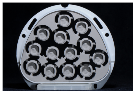
Figure 2. Milled primary crowns in the chalky blank of the Co-Cr material.
